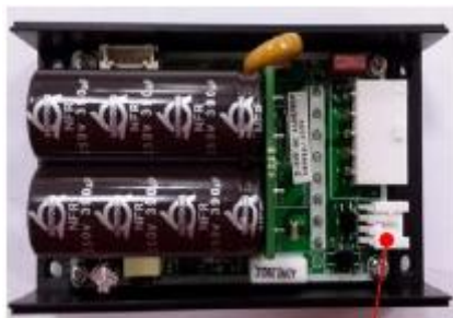
Outer LED source in Molex 53426-0310 #2 Pin
